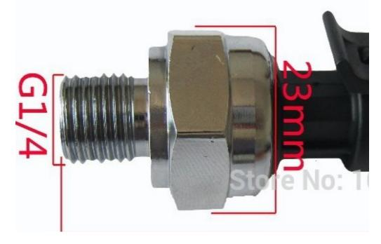
Specifications: Working Voltage: 5VDC Output Voltage: 0.5-4.5 VDC Sensor material: Carbon steel alloy Working Current:  $\leq 10$  mA Working Pressure Range: 0-30psi The Maximum Pressure: 2.4 MPa Working TEMP. Range: 0-85 degrees Storage Temperature Range: 0-100 degrees Measuring Error:  $\pm 1.5$  %FSO Temperature Range Error:  $\pm 3.5$  %FSO Response Time:  $\leq 2.0$  ms Cycle Life: 500,000 pcs Application: non-corrosive gas liquid measurement
